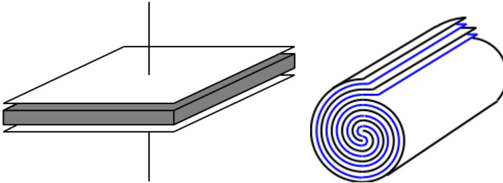
The capacitance depends upon three factors - the area of the plates ( $A$ ), the separation of the plates ( $d$ ) and the properties of the insulator represented by a constant epsilon ( $\epsilon_r$ ). The capacitance of a pair of parallel plates is given by:
