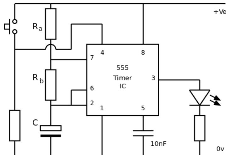
Alternatively the Astable can be controlled by a previous circuit. The system diagram below shows a Monostable with a 10 second time period (Trigger not shown) connected to an Astable with a time period of 0.5 seconds. The output of the Monostable (Pin 3) is connected to Pin 4 on the Astable. When the Monostable is triggered, the LED will flash at 2 Hz for 10 seconds. When the output from the Monostable goes LOW, the output of the Astable is reset and also goes LOW and the LED stops flashing.
