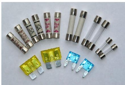
A fuse is a thin piece of wire included in a circuit. The material from which the fuse wire is made usually has a lower melting point and a slightly higher resistance than the other wires in the circuit. If too much current flows in the circuit, the fuse wire will get hot (due to its higher resistance) and melt (due to its lower melting point) before any of the other wires get hot. Once the fuse melts, the circuit is broken and no more current flows.
