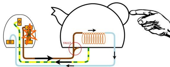
The circuit has a fault. The Live wire is touching the metal kettle and the person will receive an electric shock. However, a large current now flows along the Earth wire. This current is enough to blow the fuse and disconnect the electrical supply.
