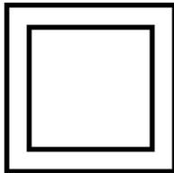
Double Insulation Symbol which represents the two separate layers of insulation rendering the Earth wire unnecessary. Double insulated often still have a fuse to prevent excess current causing a fire.
