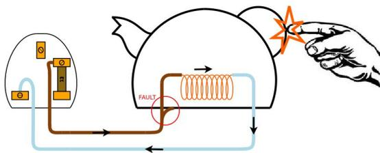
The circuit has a fault and no Earth wire. The Live wire is connected to the metal case of the kettle and the user will get an electric shock. The small extra current through the person is not enough to blow the fuse. The kettle remains connected to the electrical supply and is a danger to the user.
