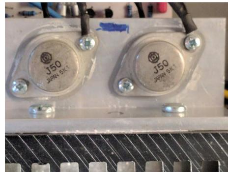
Small signal MOSFETs can be used to make amplifiers and other analogue circuits as well as making all types of digital circuits. The very high input (Gate) resistance of the MOSFET makes them ideal as input amplifiers to many devices. For example, a MOSFET is used as the input amplifier in a digital voltmeter (such as a multimeter) meaning the voltmeter has an almost infinite input resistance.
