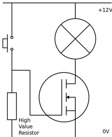
A MOSFET is very easy to use as a transducer driver because there are no other components needed and no calculations to perform. The electrical signal from a control circuit is used to control the MOSFET and the MOSFET controls the current through the output transducer. The only consideration is to make sure that the Gate-Source voltage is high enough to fully turn on the MOSFET.
