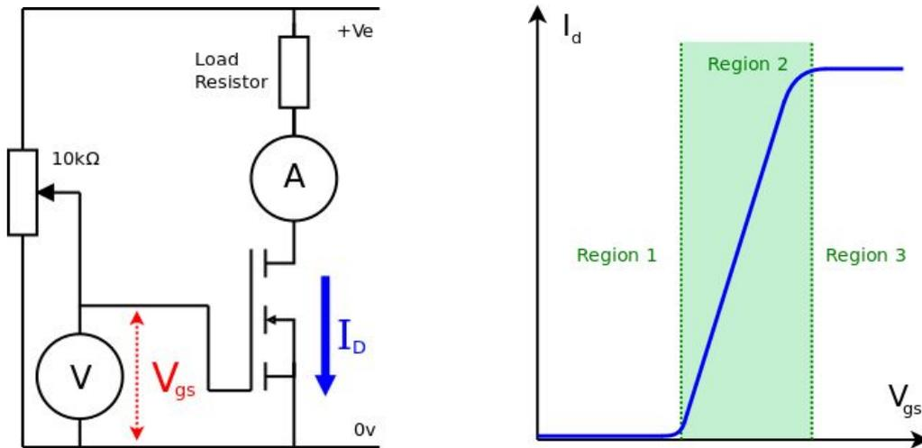
The circuit shown can be used to investigate the transfer characteristics of a MOSFET and is very similar to the circuit used to investigate the MOSFET equation. A voltmeter measures  $V_{GS}$  and an ammeter in series with a load resistor measures  $I_D$ . The addition of the load resistor limits the maximum Drain current and means the MOSFET is acting as a transducer driver with the load resistor acting as the output transducer.
