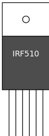
An n-channel MOSFET is an active circuit component with three legs and usually made from silicon. The n-channel MOSFET is usually just referred to as a MOSFET. A MOSFET is just one example of a Field Effect Transistor (FET) and all these devices rely on the electric field due to a voltage. MOSFETs are voltage operated devices.
