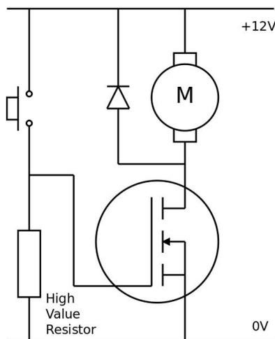
If an inductive load, such as a motor or relay, is used then a protection diode is needed to protect the MOSFET from the back EMF produced when the transducer is turned off.
