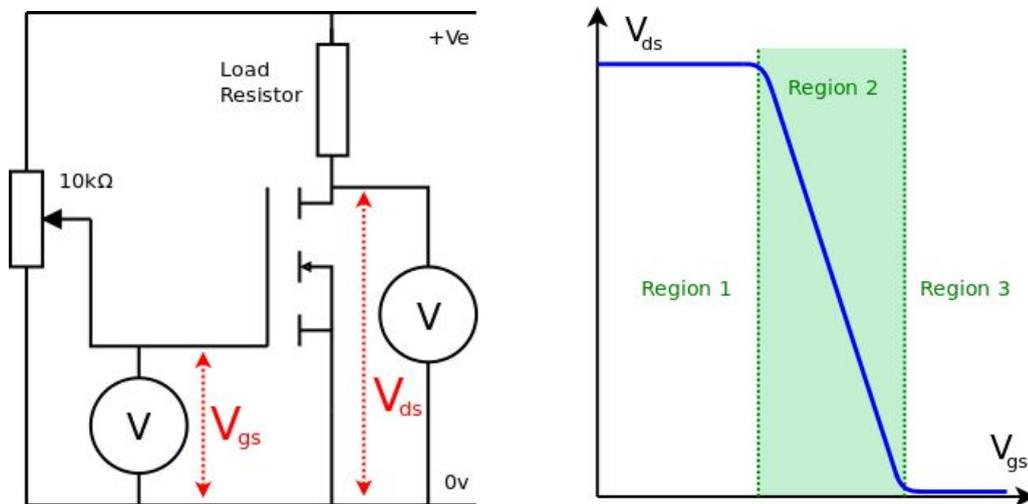
The circuit shown can be used to investigate the transfer characteristics of a MOSFET. The potentiometer allows the Gate-Source voltage to be varied.  $V_{GS}$  (sometimes called  $V_{in}$ ) and  $V_{DS}$  (sometimes called  $V_{out}$ ) are measured using voltmeters.
