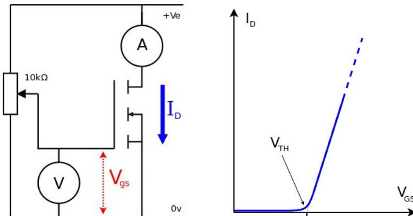
The circuit shown can be used to investigate the MOSFET equation. The potentiometer allows the  $V_{GS}$  to be varied and the ammeter measures the Drain current,  $I_D$ .
