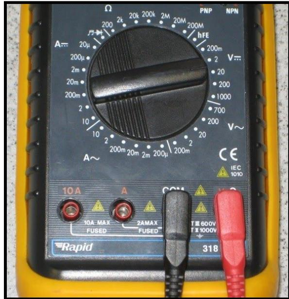
**Note:** The multimeter will measure both Potential Difference and EMF and both of these quantities are simply referred to as 'voltage' even though this is not strictly correct.
