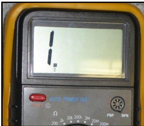
The picture shows the display you are likely to get if your multimeter is out of range. This means what you are trying to measure is bigger than the display can handle. on a 3 ½ digit display the maximum value displayed is 1999 as the 1 is the half digit. Therefore, if the meter is on the 2 V setting, any voltage above 1.999 V will display "1" - out of range
