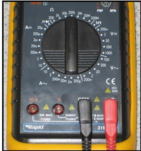
To measure resistance, connect the probe leads to COM and "Ohm" and connect the multimeter in parallel with the component being tested. As with voltage and current, the function selector should be set to the most appropriate range to give the greatest level of precision. For example, consider each of the following settings used to measure a resistance of approximately 1 k $\Omega$ :
