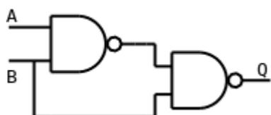
Therefore the entire circuit can be reduced to just two logic gates which can be built with **one** IC - much better.
