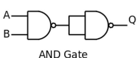
The first logic gate is the NAND gate. The second logic gate is a NOT gate which inverts the output of the NAND gate to give the output required for an AND gate.
