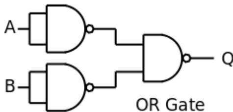
To make an OR gate, use two NAND gates as NOT gates to invert the inputs to the remaining NAND gate.
