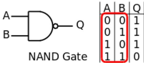
Looking at the inputs of the NAND gate it is clear that the truth table would give the correct output for an OR gate if all the inputs were inverted.
