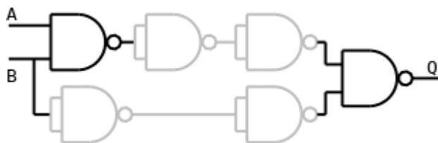
In two places a NOT gate follows a NOT gate and so these cancel and can be removed - shown in grey.
