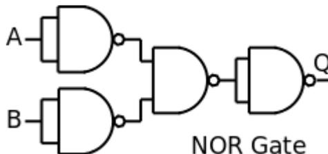
The first three logic gates make the OR gate.
