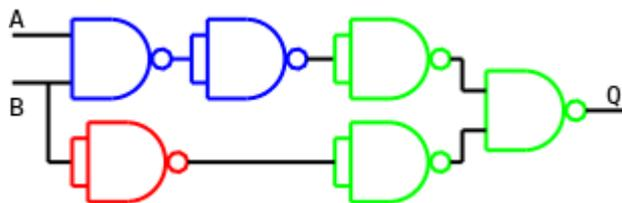
All of the logic gates are replaced with their NAND gate equivalents.
