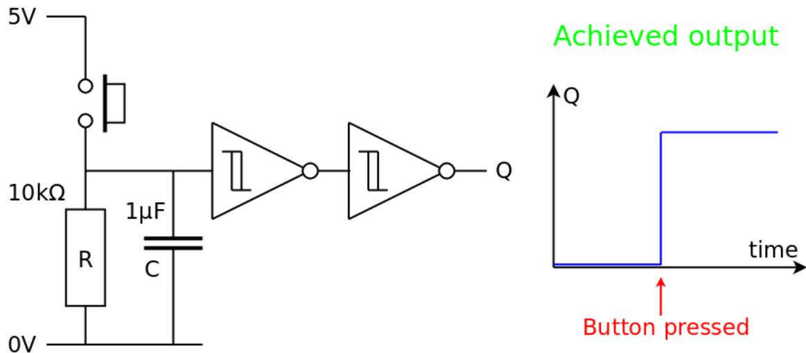
The time constant of the RC circuit must be longer than the bouncing of the contacts but short enough so that the output signal goes low almost as soon as the button is released. The Schmitt inverter is required to ensure a single clean transition as the RC circuit discharges when the push button is released. In the diagram, the second Schmitt inverter is used as a simple inverter to re-invert the output.
