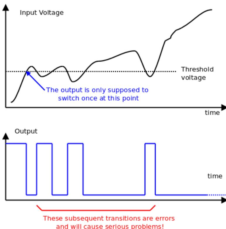
The system might be a comparator, a logic circuit or a simple NOT gate. An application of this system might be a trigger for a monostable that opens the curtains when the slowly rising light level reaches a certain brightness in the morning. The light level, and hence the input voltage, is generally increasing but fluctuates, maybe due to clouds or shadows.
