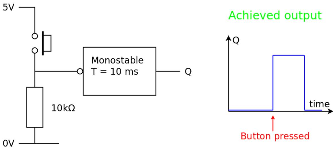
The **advantage** of using a monostable circuit is that a single clean pulse of a known duration is produced when the button is pressed. The time period of the monostable must be longer than the duration of the bounces.
