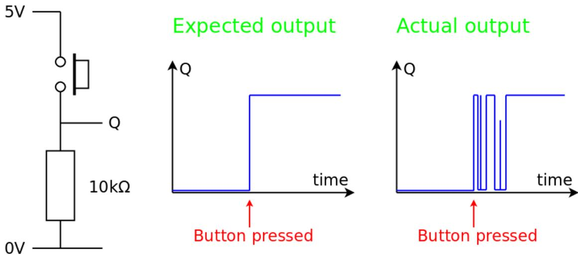
When the push button is pressed the expected output is a single clean transition from logic 0 to logic 1 but in reality several pulses may be produced as the mechanical contacts bounce.
