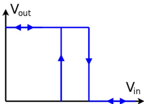
A Schmitt inverter acts like a NOT gate. The transfer characteristics show that when  $V_{in}$  is LOW (zero),  $V_{out}$  is HIGH, when  $V_{in}$  is HIGH (logic 1),  $V_{out}$  is LOW.
