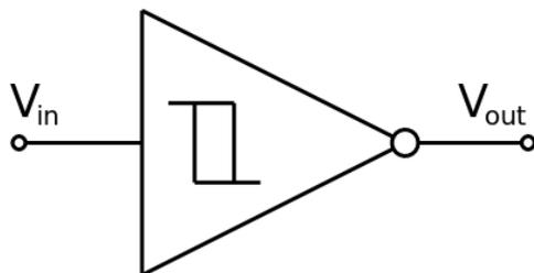
The Schmitt inverter often comes as a 14 pin IC with six inverters on one chip. The inverters can be used completely independently of each other. The hex Schmitt inverter has the same pin layout as a hex NOT gate and can be used as a direct replacement, especially when the inverter has an analogue or slowly changing input.
