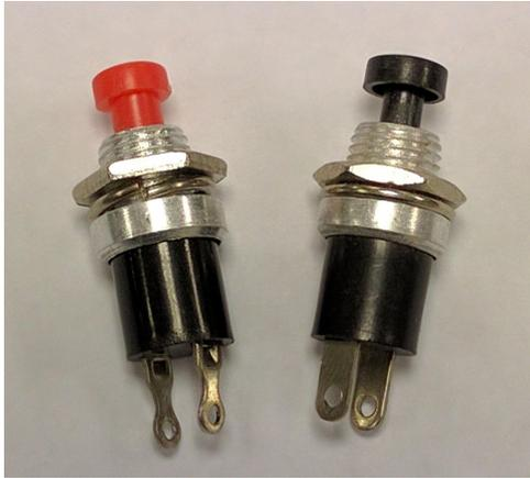
Switches and buttons can either be normally open (NO) or normally closed (NC). These are important terms to know.
