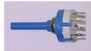
The photograph is of a stereo 6 pole rotary switch meaning there are two independent switches on the same rotary shaft, each with 6 switch positions.
