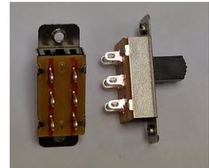
DPDT switches are also useful for routing signals in audio equipment where two separate switches are needed for the left and right stereo channels.
