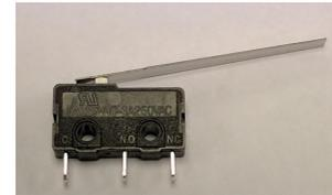
A micro switch is one that requires a very small force to operate it so that it is easy to switch. Micro switches are used in sensors and control equipment. Micro switches are spring loaded. Their normal state is when no force is applied and the switch is not activated. When a force is applied, the switch is activated. When the force is removed the switch returns to its normal state. Micro switches are more like push buttons than switches in this respect.
