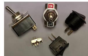
Single Pole means there is just one switch - one wire in and one wire out. On each of the switches shown there are only two contacts.
